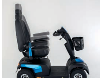
Seat riser electronically increase the seat height to achieve a preferred driving height.
